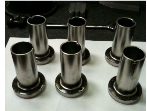
Machining (Weld and tuning margin included)
