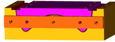
Center shell machining Weld margin included
