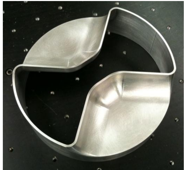
Welding cavity shoulder and center shell
