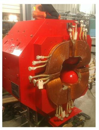
In addition to installing new coils, MAG\_TEST performed full refurbishment of both quadrupoles (sand off rust, paint, new water hoses, etc.)
