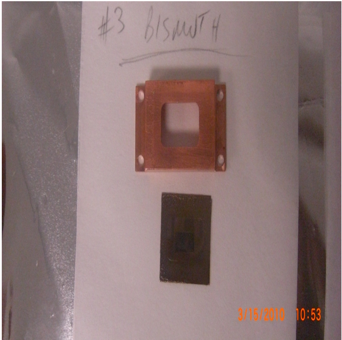
Figure 7.1: Bismuth target(0.203mm) after exposure to the beam. Discoloration on target surface is the raster pattern. Visual inspection of the bismuth target shows no significant change in the target's structure.
