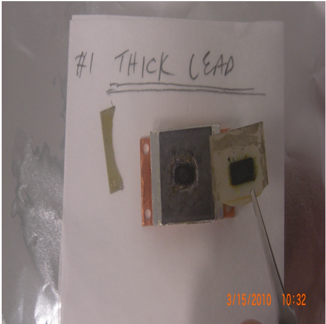
Figure 8.1: Thick lead target(0.5mm) after exposure to the beam. Visual inspection shows a significant change in the target's surface. There appears an indentation in the raster pattern with a ridge around the crater.
