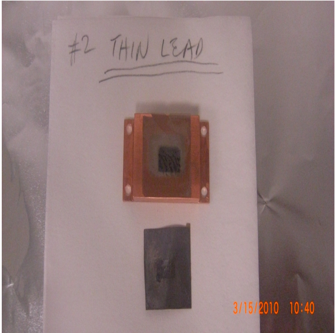
Figure 6.1: Thin lead target(0.17mm) after exposure to the beam. Discoloration on target surface shows the raster pattern. No distortion of the lead foil is seen in the visual inspection.
