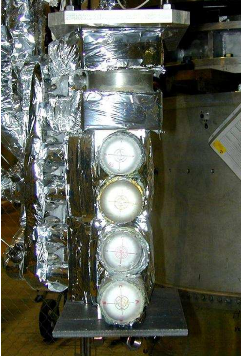
Figure 2-5: Photograph of Hall A cryogenic targets. Helium "tuna can" target is at the top of the assembly. Photograph courtesy of D. Margaziotis, CalState L. A.
