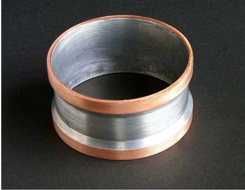
Figure 2-6: Aluminum side wall and flanges of the “tuna can” target. Photograph courtesy of D. Margaziotis, CalState LA.
