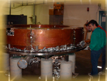
The superconducting solenoid provides a very intense magnetic field (about 2 Tesla). The magnet is actually made of 4 separate superconducting coils. The photograph here shows one of the coils being tested at the Indiana University Cyclotron Facility.
