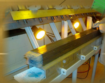
The Barrel Calorimeter is a large cylindrical detector that can measure the energy of photons or electrons. The calorimeter is made by gluing together many layers of scintillating fibers and lead. This photo shows one section being made at the University of Regina in Saskatchewan, Canada, one of a number of international collaborators on the GlueX experiment.
