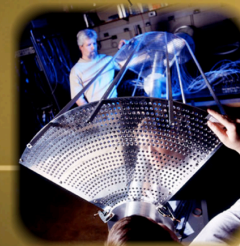
The Central Drift Chambers, like the planar drift chambers, detect electrically charged particles as they pass through. This photo shows R & D work being done at Carnegie Mellon University on a prototype. The chambers amplify small signals using gas which can be ionized and wires at high voltage.
