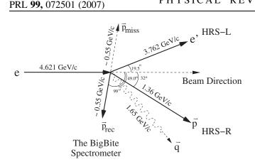
FIG. 1. A vector diagram of the layout of the  ${}^{12}C(e, e'pp)$ experiment shown for the largest  $p_{\text{miss}}$  kinematics of 0.55 GeV/c.
