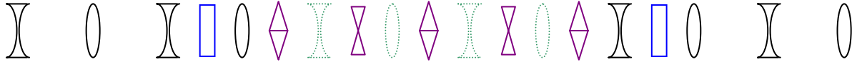
Figure 2: 3F FODO quad array during rotator operation. Center normal quads (green, ghosted) are de-excited. Additional normal quads (blue) are made available in the upstream and downstream array to support matching. Five skew quads (violet) in a symmetric FODO array are used to form the rotator.
