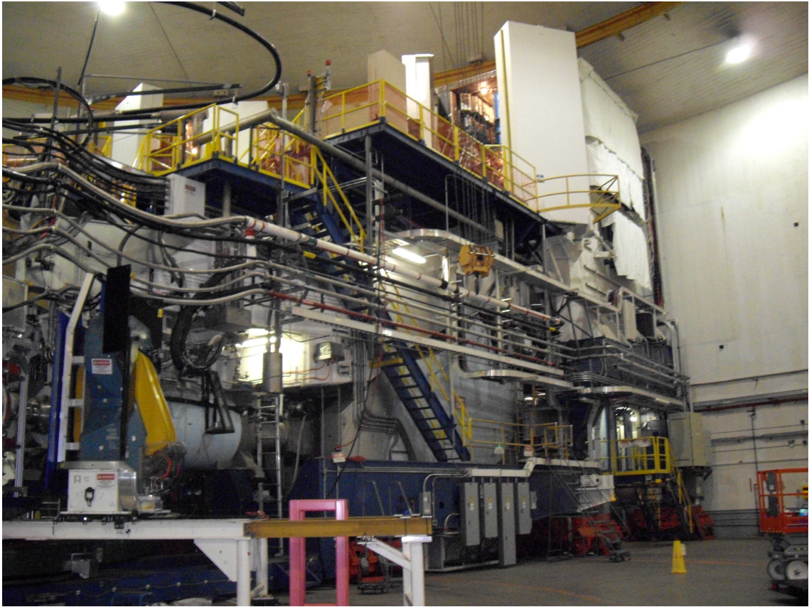
Fig. 3.17: This photograph shows the Right High Resolution Spectrometer (RHRS) in Hall A. The detector package at the top of the RHRS is outside of the shield hut. During the experiment, the detector package was in place in the hut and the doors were closed. Also visible is the BigBite magnet, painted blue and yellow to the bottom left of the photograph, which was used to detect protons and deuterons.
