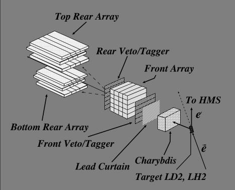
→ rotate longitudinal pol with Charybdis magnet want to determine  $P_l$  and  $P_t$  at target polarimeter sensitive to transverse pol only
