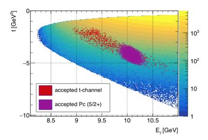
Figure 3: Full phase space of the t channel elastic  $J/\Psi$  production with the acceptance rate shown. The variable t versus incoming photon energy  $E_{\gamma}$  is plotted. The kinematic setting (# 1) for this experiment with the accepted t channel events (red) and the  $P_c(4450)-5/2+$  (purple) resonant state events.
