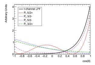
Figure 5: Angular distribution of the  $J/\Psi$  production for the t-channel, normalized to the same area for each curve in arbitrary units, in comparison with the  $J/\Psi$  production through the exotic  $P_c$  resonant state with various possible spin/parity assumptions. Note that, for the t-channel this is directly related to the t-dependence of the cross section.
