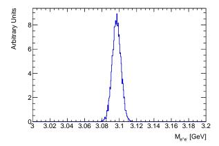
Figure 11: Invariant mass of the detected lepton pair with realistic smearing. The full width at half maximum of the spectrum is 12 MeV.
