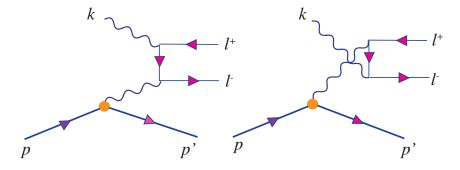
Figure 8: Bethe-Heitler (BH) mechanism producing a background process to the t-channel and  $P_c$  resonant production.
