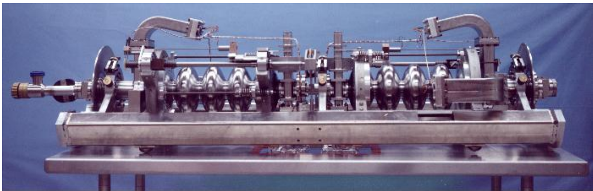
Figure 3-2: A pair of the standard five-cell Niobium accelerating cavities used in CEBAF.
