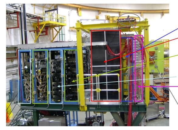
Lead Glass 1744 blocks (4300kg) Black Box (PMs, bases, patch boards, temperature & door sensors) Front-End Electronics (incl. trigger) Booster Power Supplies Signal Patch Panels HV Patch Panels Light Box (monitoring system) Scintillators (for cosmics) Absorber (4" Al)
