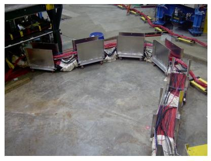
1782 + 82 signal cables (100m) for ADC
