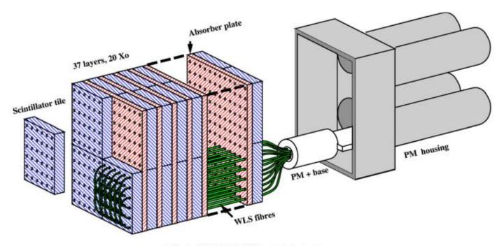
Fig. 4. MIDDLE ECAL module structure.
