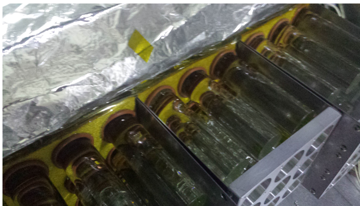
Figure 9: Rear heating of block stack with partition implementation.
