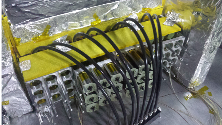
Figure 23: Rear heating of block stack with 1/4" tube 8-way manifold cooling near the partition.
