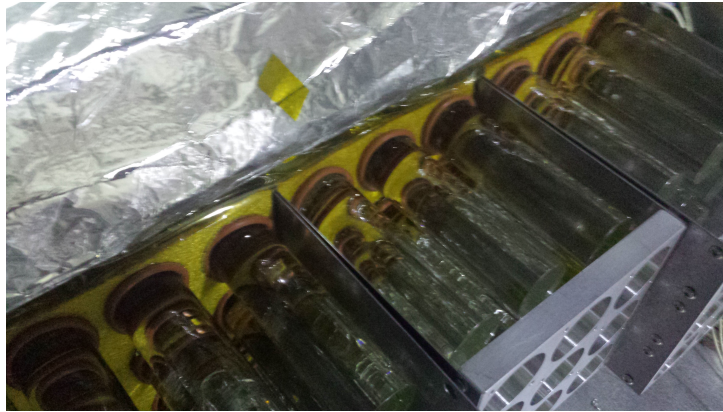
Figure 16: Rear heating of block stack with partition implementation in C200.
