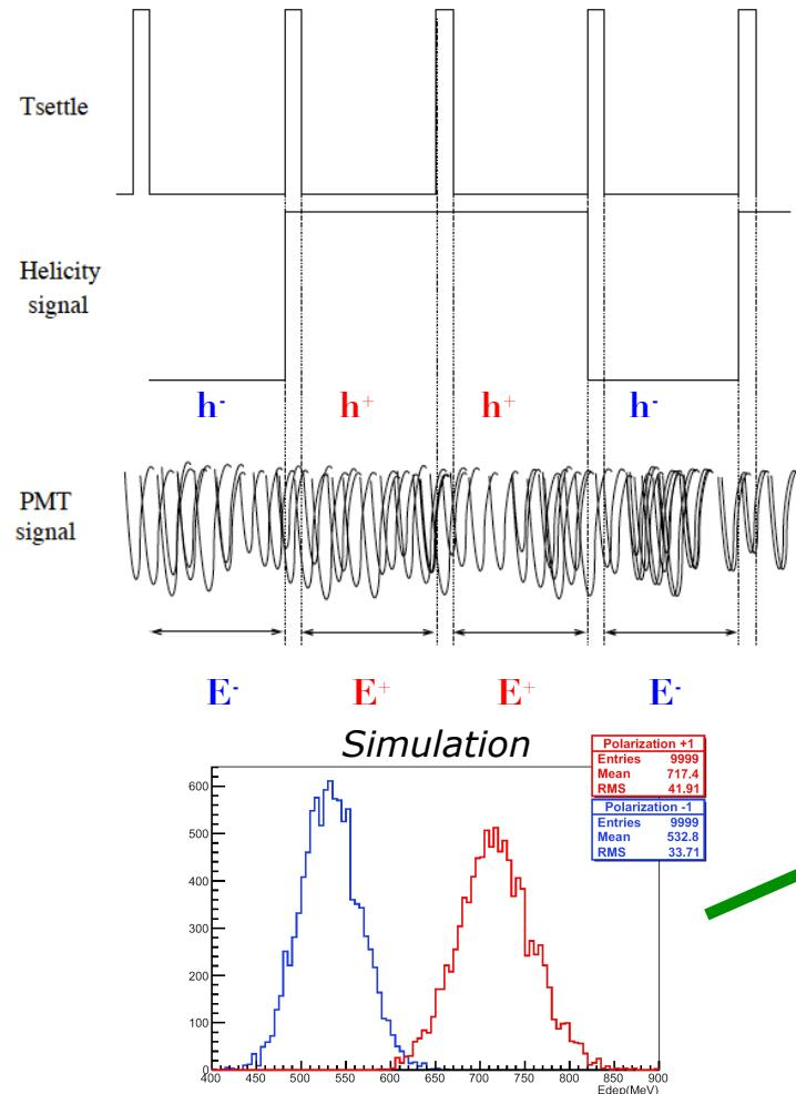
➤ The **integrated mode** operates for **high rate** conditions by **integration** of the **PMT signal** over the duration of an **helicity gate** (PEPPo firmware developed by JLab).
