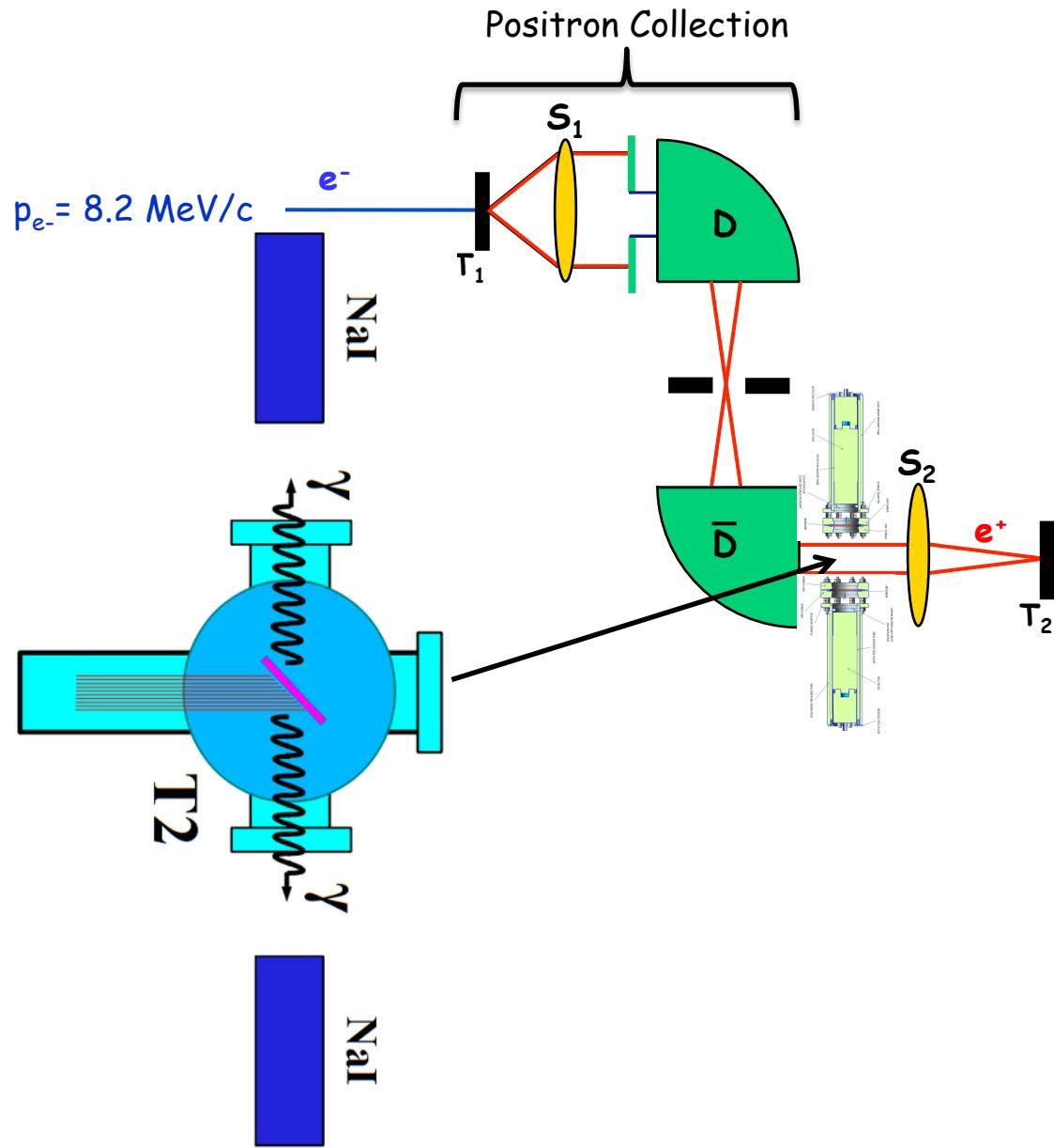
The positrons produced in the PEPPo experiment are detected using a set of two annihilation counters. The positrons stopped in an insertable 0.011" chromox target and the corresponding 511keV photons detected in coincidence with two NaI detectors.
