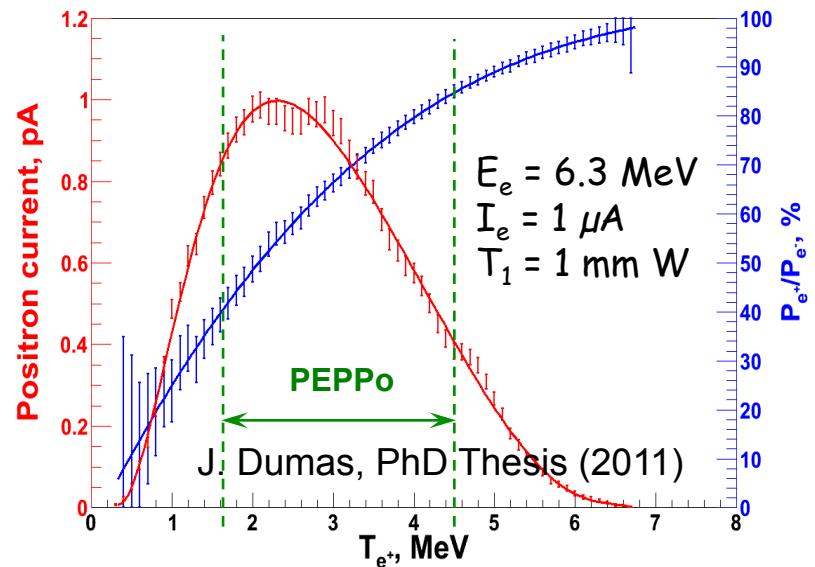
PEPPo measured the polarization transfer from 8.2 MeV/c longitudinal electrons to longitudinal positrons in the 3.1-6.2 MeV/c momentum range.
