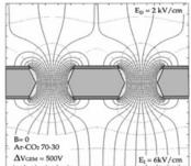
When a voltage difference around 400 V is applied on both side of the GEM foil, an electric field as high as 100 kV/cm will be created in the holes and result in the charge amplification
