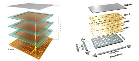
• A photolithography and acid etching process makes 30–50 µm diameter holes through both copper layers; a second etching process extends these holes all the way through the kapton.
