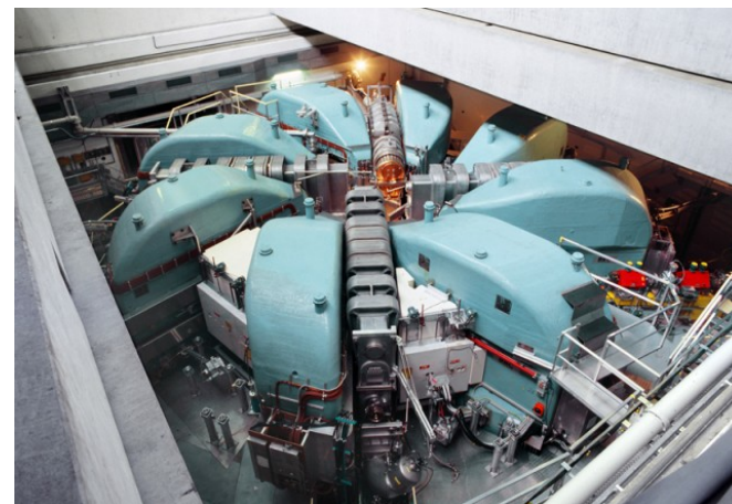
The proton accelerator at the Paul Scherrer Institute, which was used to create the muons used in this experiment. Paul Scherrer Institute
