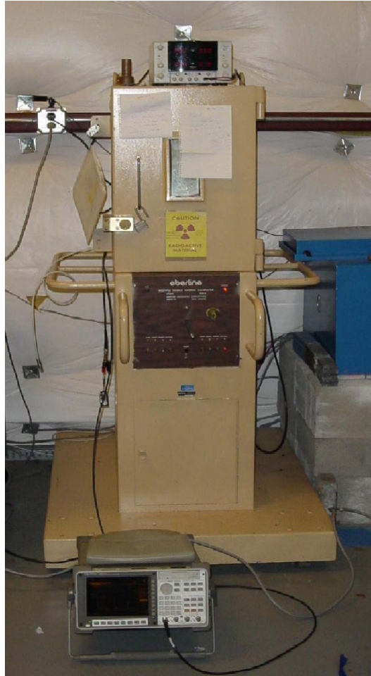
Figure 2: ^{137}\text{Cs} irradiation facility location in the RadCon test range. The top opens like a refrigerator in which samples can be placed on shelves for irradiation. The ^{137}\text{Cs} source is located in the bottom section. On top of the irradiator is our regulated DC power supply, and sitting in front of it is our spectrum analyzer.
