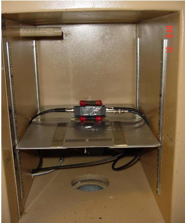
Figure 3: The box in which samples are irradiated. When the door is closed and the shutter is opened, \gamma 's are emitted from the hole in the bottom. Dosimeters are visible above and below the preamplifier.
