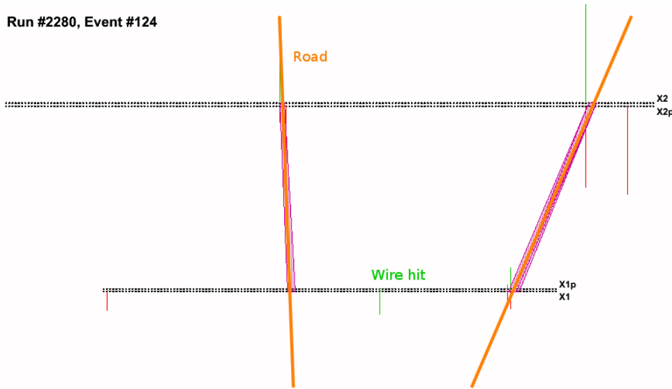
Figure 3.37 — Reconstructed two-dimensional tracks (roads) in the x -projection of MWDCs. Each projection combines four wire planes (e.g. x1 , x1p , x2 , x2p ). Wire hits in each plane are shown with red and green vertical lines. The length of a line corresponds to the distance (not in scale) from the wire. Hits from all wires are introduced to the Pattern Match Tree Search algorithm which finds possible roads. The roads from all three projections ( x , u , v ) are then combined into three-dimensional tracks.
