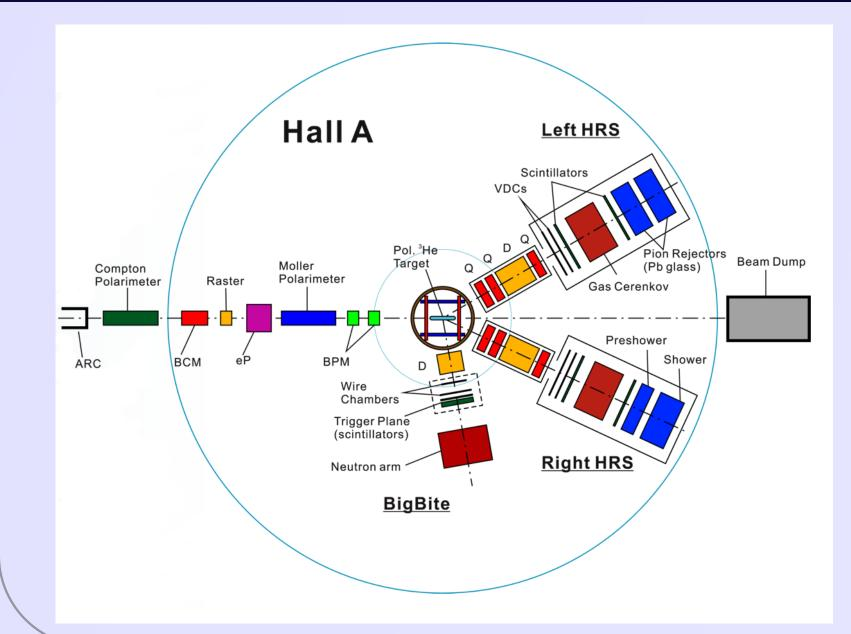
The instrumentation in Hall A [4] was designed to study electro- and photo-induced reactions at very high luminosity and good momentum and angular resolution. The central components of Hall A are two high-resolution spectrometers with the momentum resolution better than  $2 \times 10^{-4}$ . The research program is aimed at a variety of subjects, including nucleon form factors, nucleon electromagnetic and spin structure fuctions, and properties of the nuclear medium.
