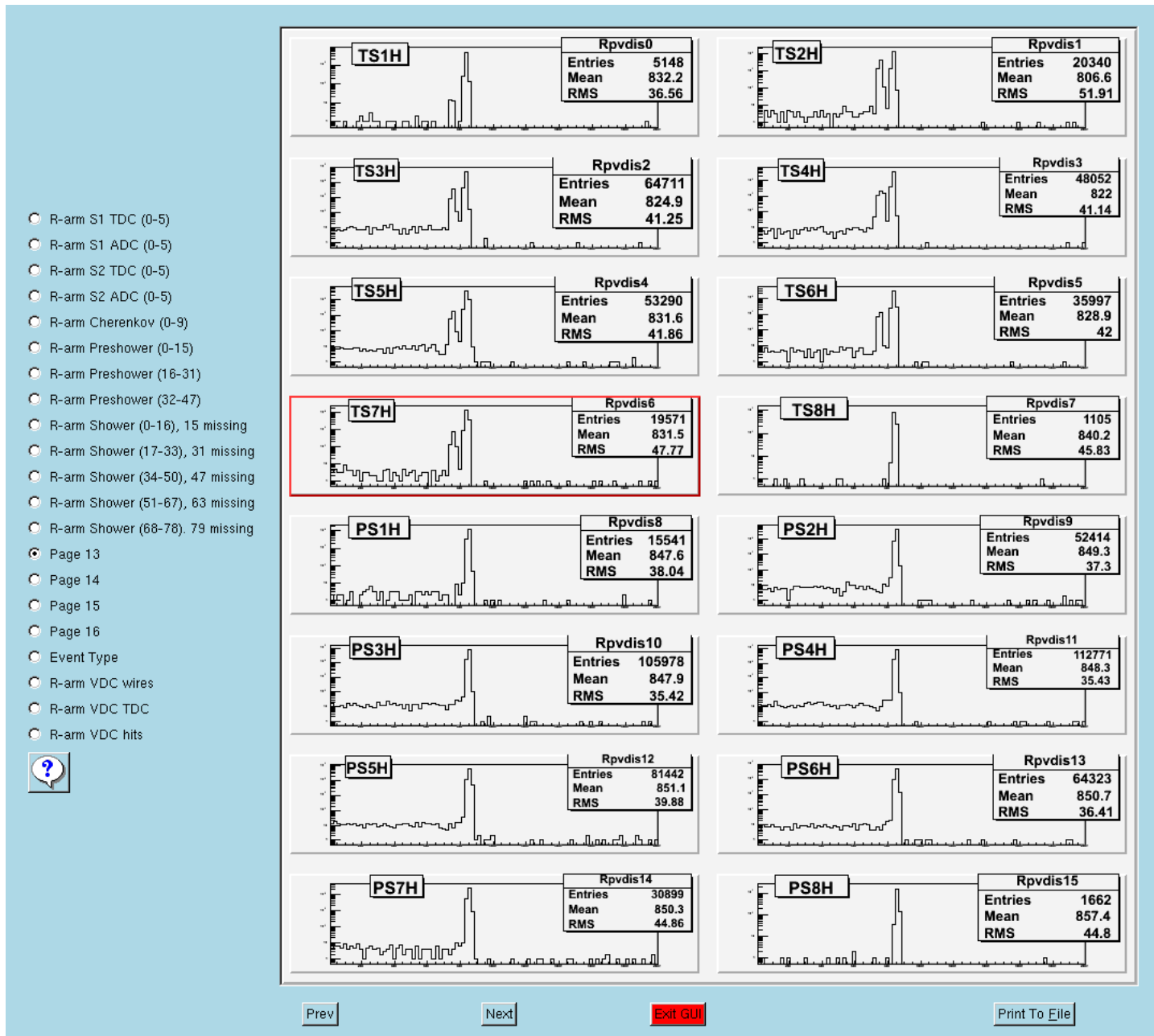
Figure 1: Fastbus 1877 TDC 1 to 16. The title in the plot shows which TDC channel has which signal from the PVDIS flow-chart-diagram. The TDC was in common-stop mode. The common-stop for these data was provided by only T1 (S1 .and. S2)-trigger. The rightmost peak in the TDC-histogram belongs to an EDTM pulser signal. Any trace left to the EDTM signal is the signal due to PVDIS triggers.
