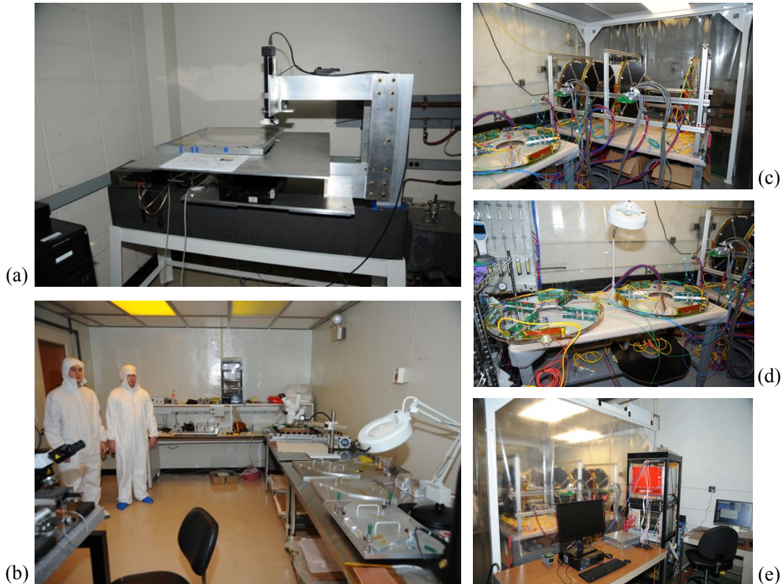
Figure 2: Complete GEM lab infrastructure at Temple University in the current Department of Physics showing a dedicated clean room for assembly and testing (b), the CCD-camera optical scanning table (a) and the actual GEM testing lab (c-e).
