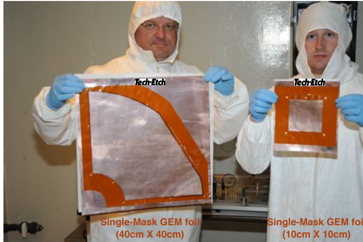
Figure 4: Photograph of two single-mask produced GEM foils showing B. Surrow holding a large 40 \times 40 \text{ cm}^2 GEM foil and M. Posik holding a small 10 \times 10 \text{ cm}^2 GEM foil inside the permanent Class 1,000 clean room in the current Department of Physics.
