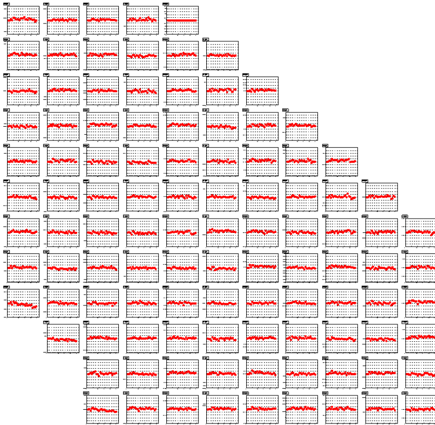
FIG. 5: Gain variations for each IC crystal in the upper right quadrant, as a function of time over the whole run, as measured by the laser monitoring system. Dashed horizontal lines are separated by 5%.
