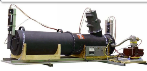
“Bazooka” LGC prototype with MaPMT
