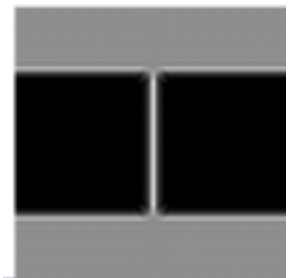
NFXrL printing of a bridge from mask (top) with width 100 nm, and resulting print (bottom) with width 33 nm. Gap 5 \mu\text{m} , \lambda=0.62\text{-}1.24\text{ nm} .
