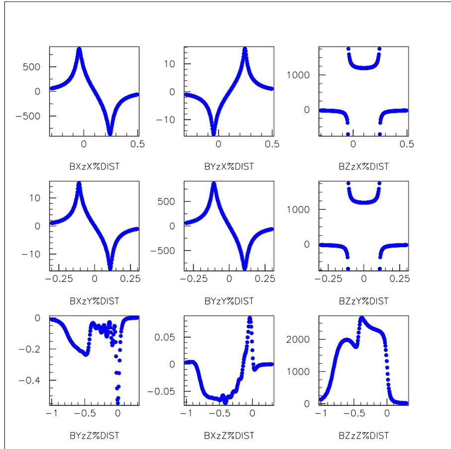
Figure 4: Fields from the transfer magnet model. Fields are in Gauss and distances are in meter. We assume a 16 A current in the coil. Top row, from left to right:  $B_x(x)$ ,  $B_y(x)$  and  $B_z(x)$  measured for  $y = 0$  and  $z = -80$  cm. Middle row, from left to right:  $B_x(y)$ ,  $B_y(y)$  and  $B_z(y)$  measured for  $x = 0$  and  $z = -80$  cm. Bottom row, from left to right:  $B_x(z)$ ,  $B_y(z)$  and  $B_z(z)$  measured for  $x = y = 0$ .
