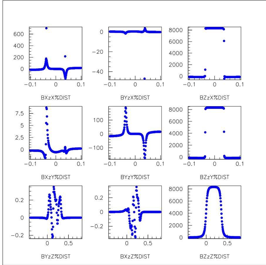
Figure 5: Fields from the main IBC magnet. Fields are in Gauss and distances are in meter. Top row, from left to right:  $B_x(x)$ ,  $B_y(x)$  and  $B_z(x)$  measured for  $y = 0$  and  $z = 20$  cm (20 cm = middle of the solenoid). Middle row, from left to right:  $B_x(y)$ ,  $B_y(y)$  and  $B_z(y)$  measured for  $x = 0$  and  $z = 20$  cm. Bottom row, from left to right:  $B_x(z)$ ,  $B_y(z)$  and  $B_z(z)$  measured for  $x = y = 0$ .
