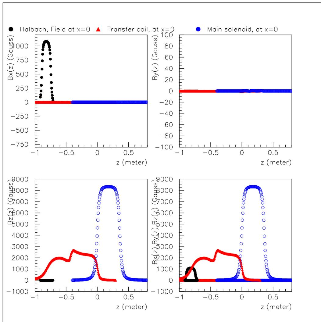
Figure 6: Fields along the  $z$  direction and for  $x = y = 0$  from the 3 magnets . Black is for the Halbach dipole, red for the transfer magnet and blue for the main IBC solenoid. The top left plot is for  $B_x(z)$ , the top right for  $B_y(z)$ , the bottom left is for  $B_z(z)$ . The bottom right panel displays all the field components on the same scale (fields components are not added).
