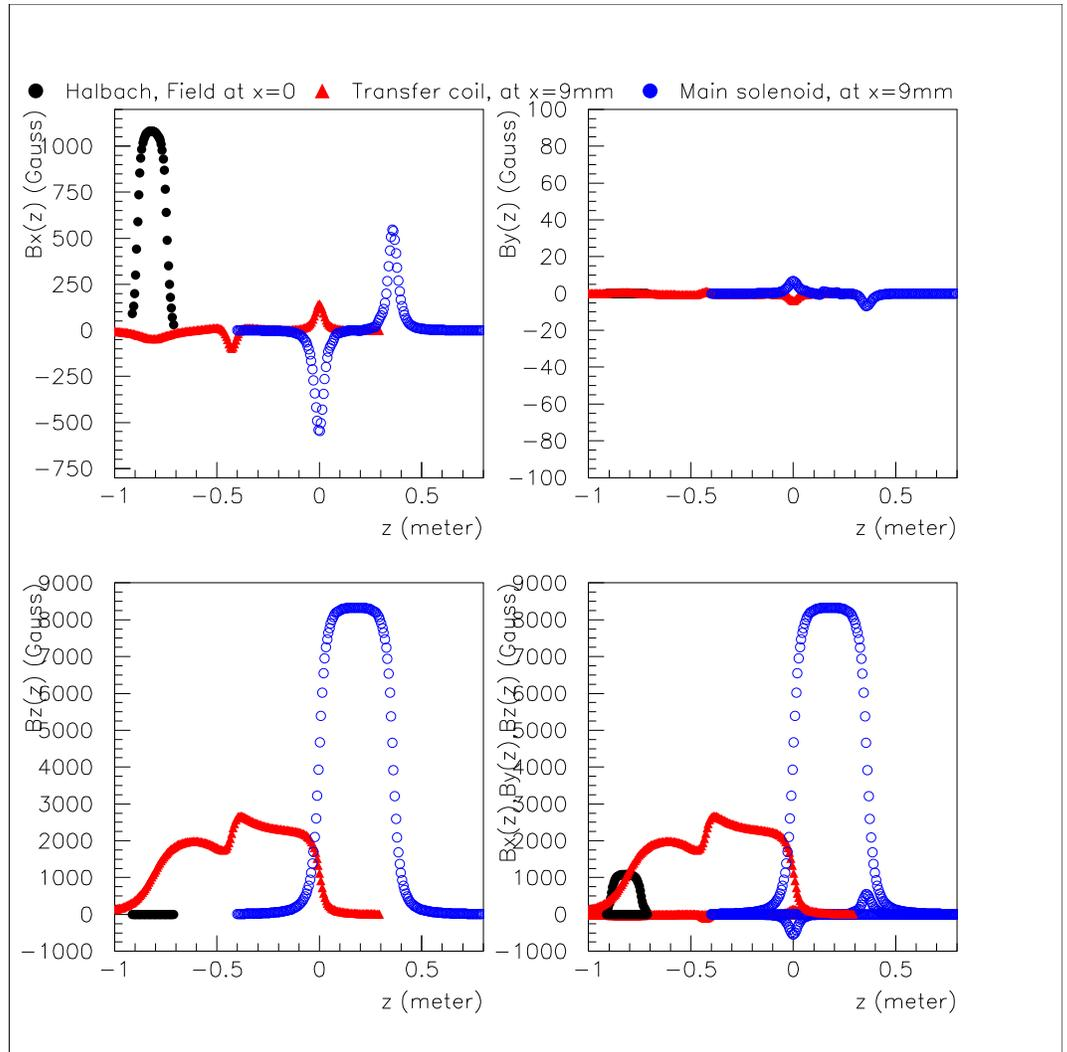
Figure 7: Same as Fig. 6 except  $x = 9\text{ mm}$  for the transfer magnet and main IBC solenoid. The Halbach field map is still at  $x = y = 0$ .
