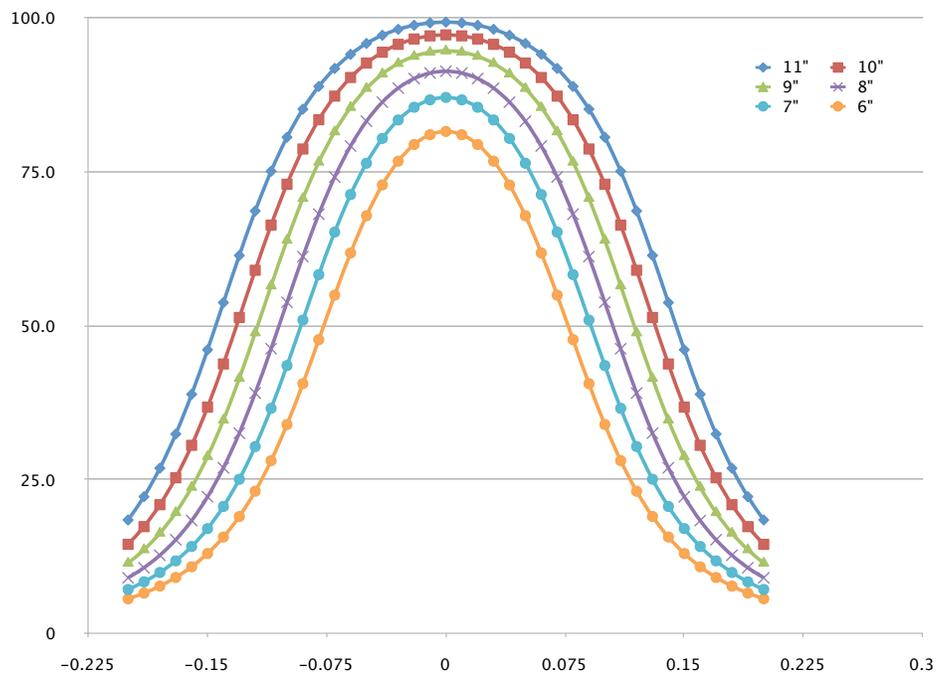
Magnetic field for different rrlength of the safety coils. The current assumed is 4.5 A for 2 layers of wire.
