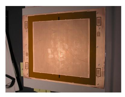
Figure 4.8: A custom 20 cm  $\times$  17 cm GEM foil, manufactured for this experiment by Tech-Etch. Fingerprints are clearly visible on the surface.
