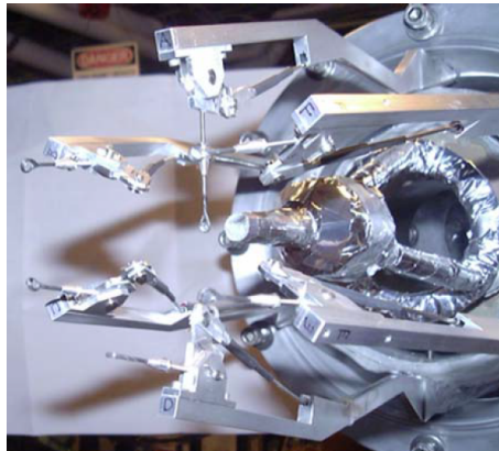
Figure 2.9: Eg2's double target system. The claws holds the interchangeable solid targets. The cylinder-shaped object wrapped in foil is the liquid target.
