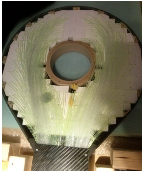
Figure 3.32 The hodoscope with the ^{207}\text{Bi} source placed on one of its tiles in the dense, but reachable, fibre area.
