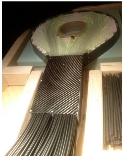
Figure 3.24 The constructed hodoscope, without the upper lid.
