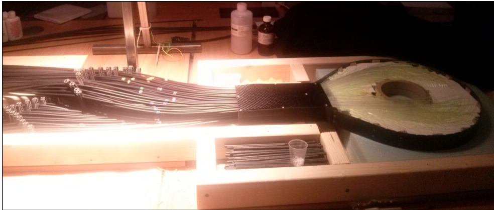
Figure 3.23 The constructed hodoscope at the Edinburgh nuclear physics group lab (the light in the lab was non-UV, and hence it wasn't harmful for the scintillators).
