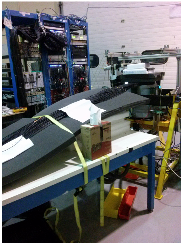
Figure 3.39 Cosmic test setup at JLab with the FT-Hodoscope and the FT-Calorimeter in vertical position. An improvised structure for holding the FT-Hodoscope fibres is shown, as well as the fADCs system for data acquisition.
