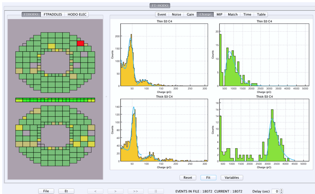
Figure 3.41 “Charge” tab of the monitoring software that shows SiPM noise histograms (yellow) and charge histograms (green), for the front (thin) and the corresponding back (thick) hodoscope tiles. The charge histograms represent the energy deposited by cosmic rays in the scintillators, and they are fitted with Landau function.
