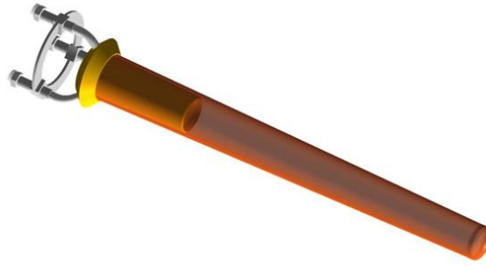
Figure 2.3 The g11a target cell, that was also used in other experiments at Jefferson Lab [38].
