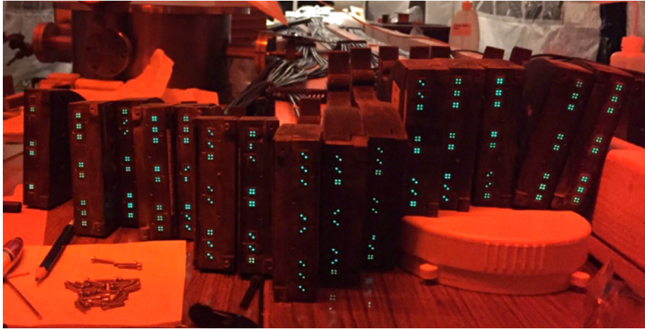
Figure 3.26 Prepared, polished optical connectors for one of the hodoscope layers. Since the hodoscope wasn't covered and the non-UV light in the lab was on, the green light was coming from the WLS fibres that were glued inside the tiles.
