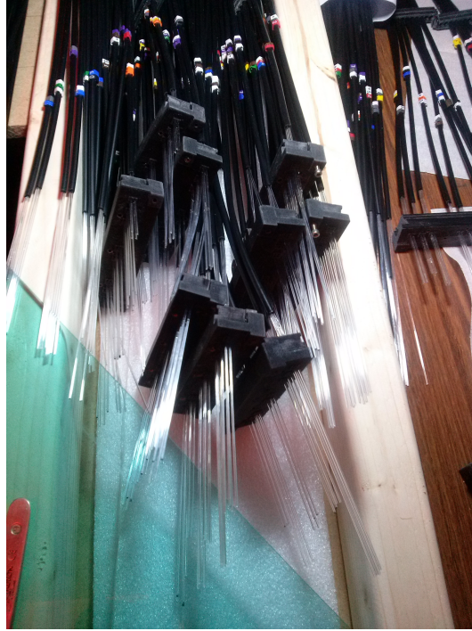
Figure 3.25 Parts of the “fish tails” with clear fibres glued inside.
