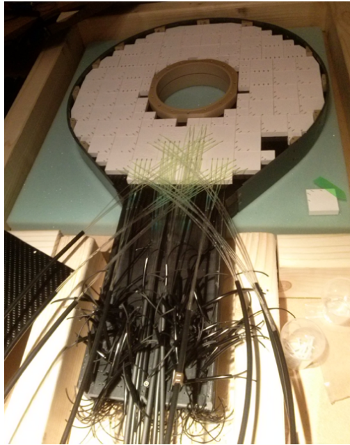
Figure 3.21 Beginning of gluing the fibres inside the scintillators, following the previously established fibre routing scheme.
