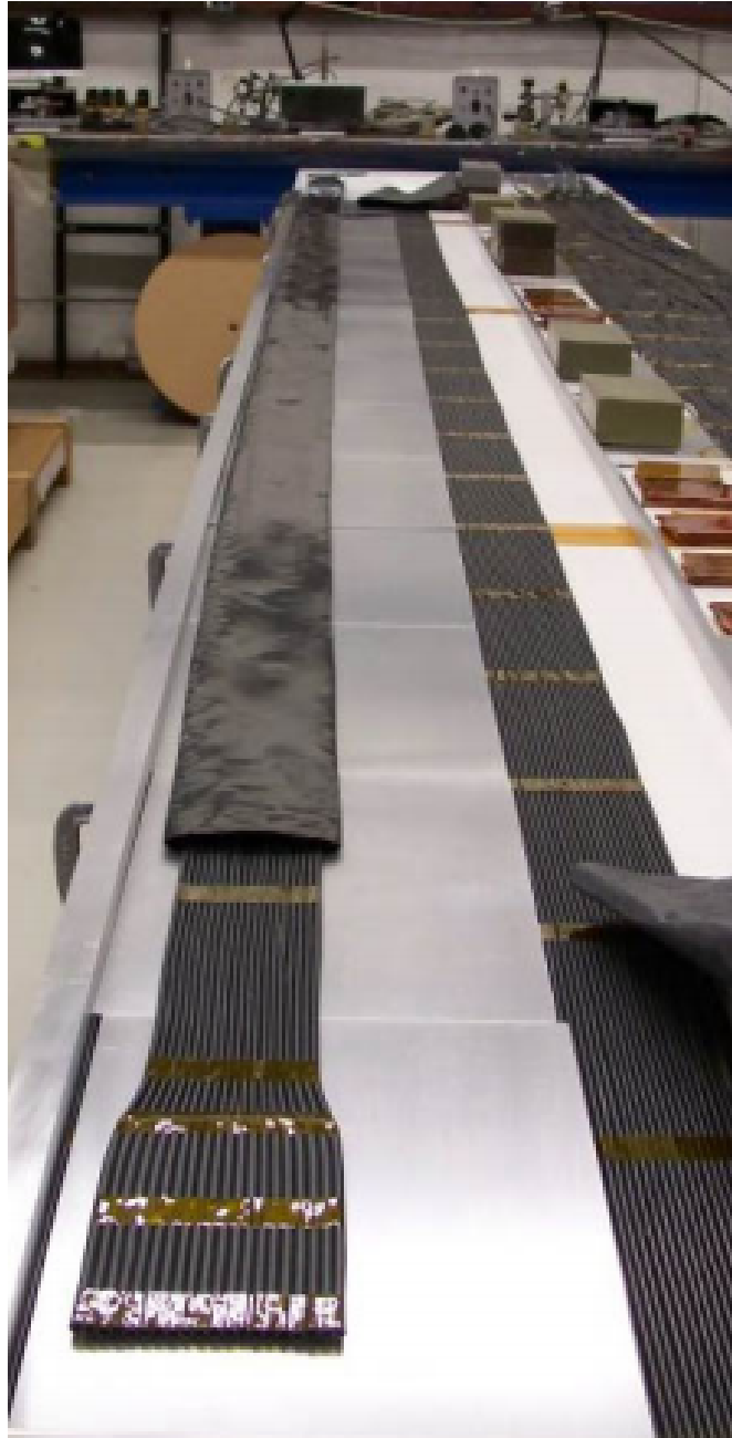
Figure 4.3 A photograph of the full length spliced fibres, with protective sheeting, after fusion splicing at Fermilab. The fibres are put into groups of 4 and placed into protective black PVC sheathing to shield them from sources of UV light.
