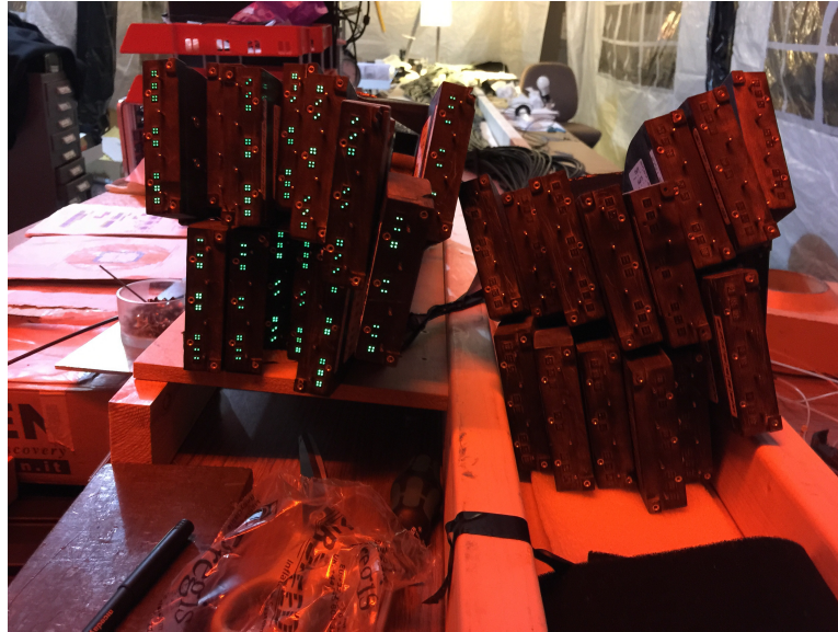
Figure 8.6 Ends of the fishtail connections after the fibres were glued into place then polished. The connectors from the layer of the Hodoscope which is currently open are clearly differentiated by the captured green light which is radiating from the ends of the connectors.
