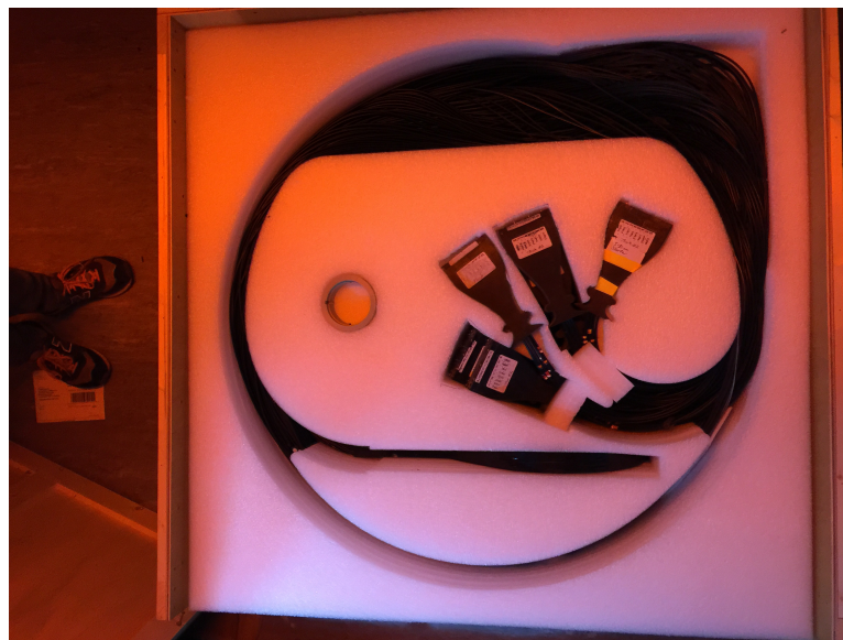
Figure 8.8 The specially designed transport crate for the FT-Hodo. Top: A CAD picture of the design. Lower: An overhead view of the FT-Hodo packed before being sealed and transported to Jefferson Lab.
