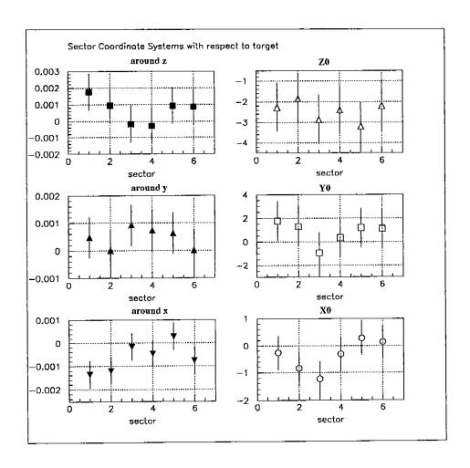
Figure 5: The rotations and displacements of the drift chambers in Sector Coordinate Systems relative to the target position. The calculation of the rotation angles and offsets for the sectors 2 and 3 is based on the three survey target locations, meanwhile for the rest of the sectors it's based on the four survey target locations. The large uncertainties for  $X_0$ ,  $Y_0$  and  $Z_0$  are due to the angle uncertainties.
