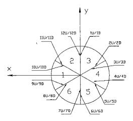
Figure 1: Schematic view of the CLAS looking downstream. The numbers 1-6 refer to the sector number; the numbers 1U/1D - 12U/12D refer to endplate survey locations.
