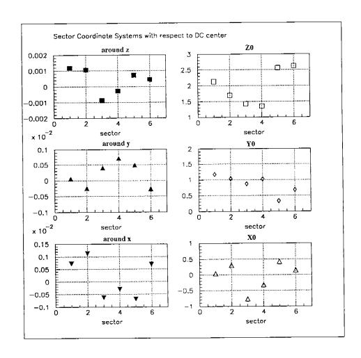
Figure 4: The rotations and displacements of the drift chambers in Sector Coordinate Systems relative to the center of the drift chamber. Rotations are calculated about the center of the 4 survey targets so as not to introduce artificial translations. The uncertainties for  $X_0$ ,  $Y_0$  and  $Z_0$  are about 0.25 mm.
