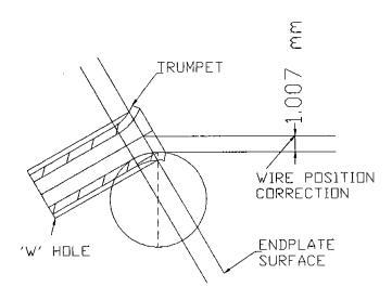
Figure 6: The wire position correction for Region 2 Drift Chambers. The 'W' hole is the wire hole. The trumpet is the metal insert. The circle has the same radius and center as the arc of the trumpet.
