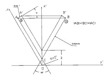
Figure 2: 2D endplate coordinate system to 3D TCS system transformation. The XY axes are in the 2D endplate system (XY axes are different for the two endplates). The X',Y',Z' axes are in the TCS system. X and Z' are directed into the page, increasing in the downstream direction (along the beam). Y is parallel to the endplate.
