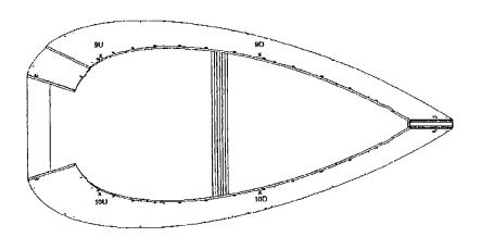
Figure 3: View on the Sector 1 from the Sector 4 drift chamber . 9U,9D,10U,10D - are the survey targets.
