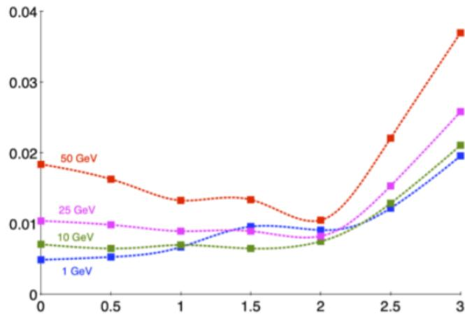
Figure 9: Momentum resolutions versus pseudo-rapidity  $\eta$  for different particle momenta.
