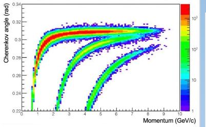
Left: hadron separation provided by RICH Right: check with semi-inclusive channel  $ep \rightarrow e'H^+X$
