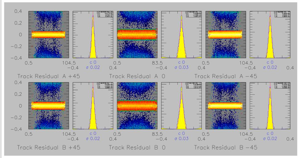
Residuals:  $x_{\text{track}} - x_{\text{hit}}^{\text{drift}}$
