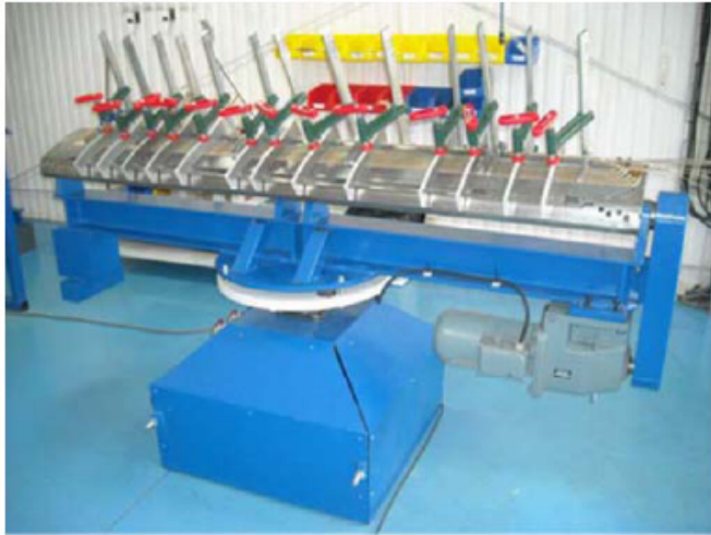
Existing 2 axis winding table for SHMS prototyping
