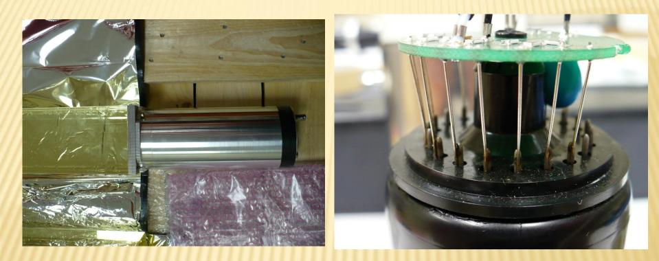
The pre-assembley studies showed all PMTs are glued to lead blocks, and HV dividers are soldered directly to PMT's. This makes technically <u>impossible</u> to change the PMT or HV base, in case of problem in the course of running experiment.
