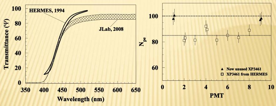
Light transmittance test for HERMES F-101 lead glass blocks. The difference between 1994 and 2008 is due to different measuring setup. Relative quantum efficiency tests of XP3461 PMTs from HEREMES. A 15% (marginal) degradation was detected.
