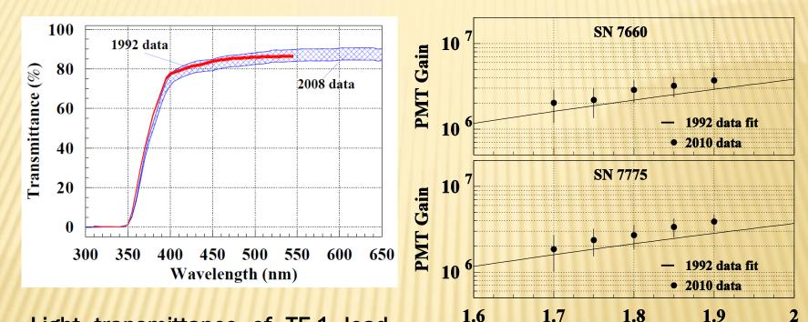
Light transmittance of TF-1 lead glass blocks, before and after use in SOS calorimeter. Signs of marginal degradation from radiation.
