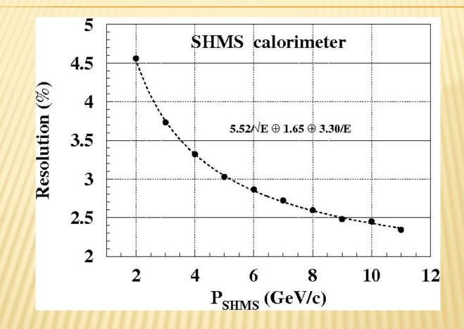
Based on MC studies the EM calorimeter resolution is similar to other lead glass calorimeters
