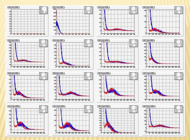
•fADC-250 are used for signal readout for Shower•The cosmic test was done by applying 1500V on all Shower blocks
