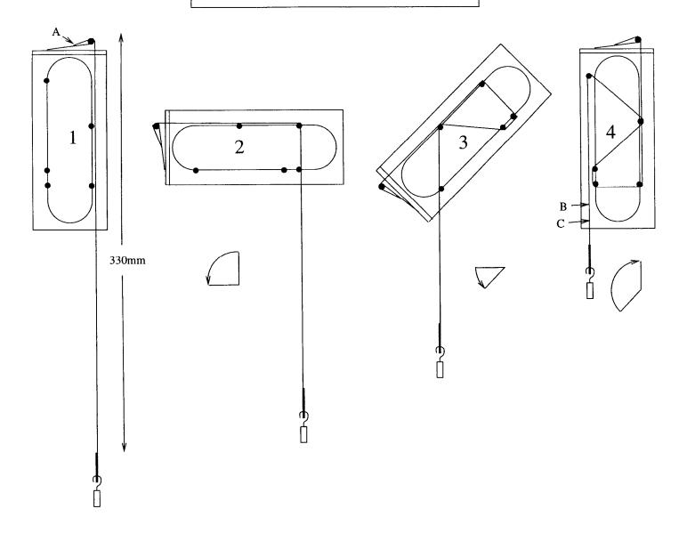
Mount the cartridge on the special tool, allowing the cartridge to rotate around a horizontal axis (Fig.1).
