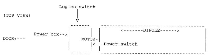
It is important NOT to switch off the logics (some data in memory will be lost), but to switch off the motor power (see the exact Power switch location above) pr to any intervention on the mechanics.
