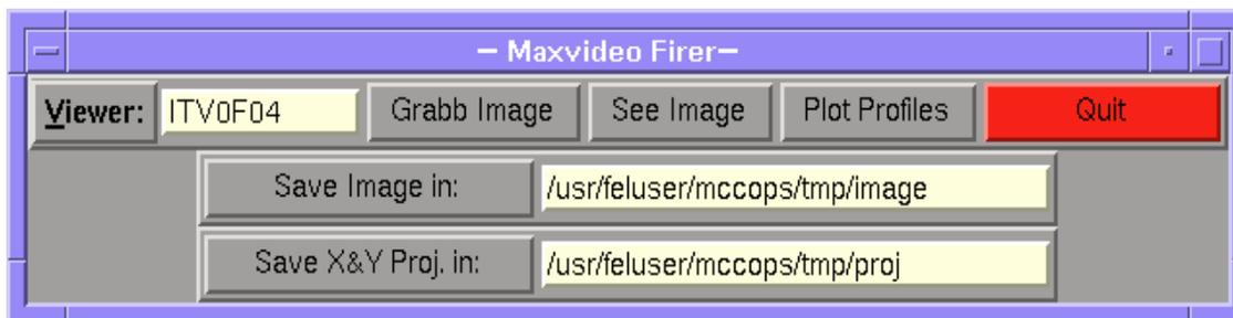
from the Viewer menu button select the viewer you are currently looking at (note that the viewer with the (OK) mentions are the one you could use i.e. the calibration has been downloaded, for the one with no OK mentioned, it has not been done because of HARDWARE mis-functions).
