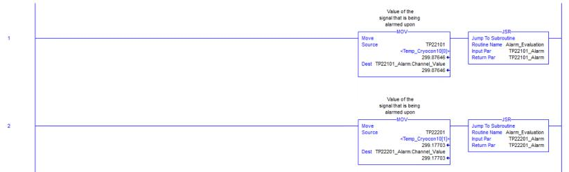
Example: If system alarms on pressure PT71010 then the tag associated with high alarm setpoint will be PT71010HiHi and for low pressure alarm set point it will be PT71010LoLo. While PT71010\_Alarm.Status will be an actual interger which will represent which level (Hi,HiHi,Lo,LoLo) of alarm is active.
