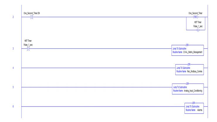
**Example:** FlowCalculation sub-routine is not requested from the MainRoutine but when Main Routine executes Analog\_Input\_Conditioning it request FlowCalculation sub-routine indirectly and executes it.
