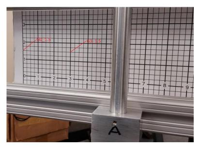
For the Secondary screen, points were considered at the intersection of the 8th horizontal line and every 10th vertical line.
