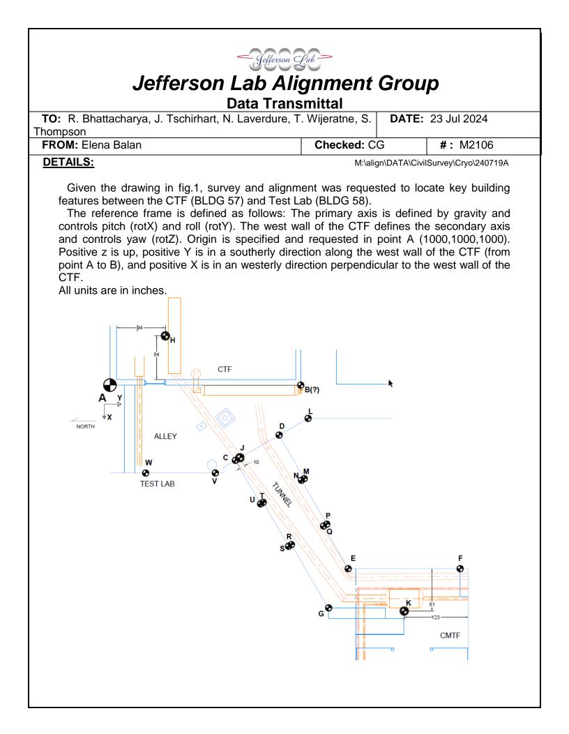
In addition to the requested features, points L through W are building corners measured and added to the drawing.
