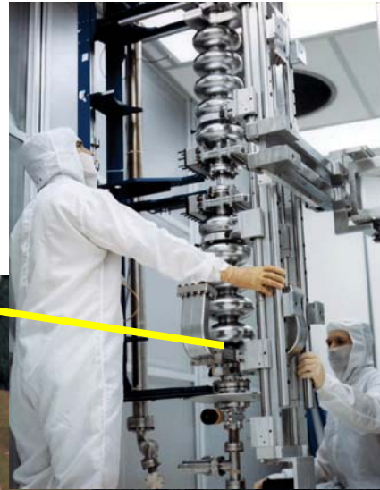
Superconducting radiofrequency (SRF) cavities undergo vertical testing.
