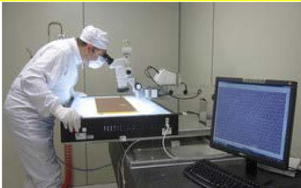
The GEM foils are tested in a  $N_2$  flushed box for humidity reduction (RH below **10%**)
