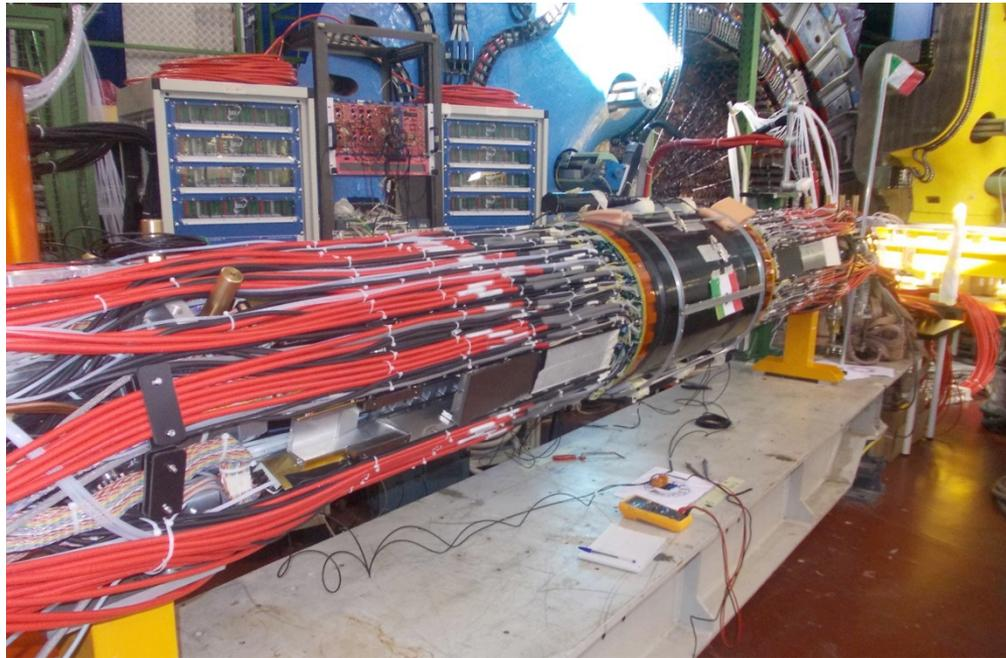
Faraday cage completed with a **18  $\mu\text{m}$**  shield connected to the PCB end caps
