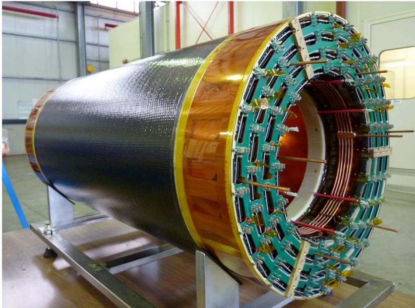
The final assembly of the KLOE-2 Inner Tracker, with the insertion of all the triple-CGEMs one into the other took place in March 2013
