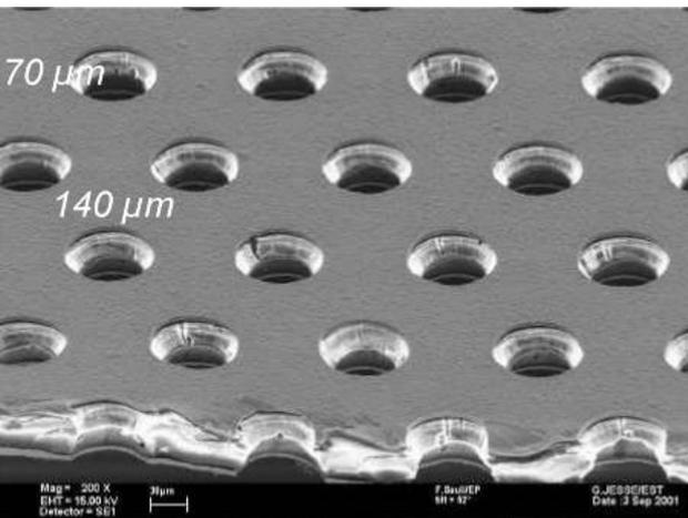
A Triple-GEM detector is built by inserting three GEM foils between two planar electrodes, which act as the cathode and the anode.
