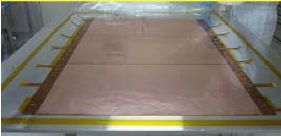
Three foils are spliced together along the kapton frame
