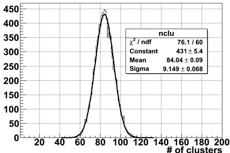
Ionization in 3 mm of Ar:CO<sub>2</sub> 70:30,  $\beta\gamma=2.21$
