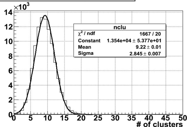
Ionization in 3 mm Ar:isoC<sub>4</sub>H<sub>10</sub> 90:10,  $\beta\gamma=0.26$
