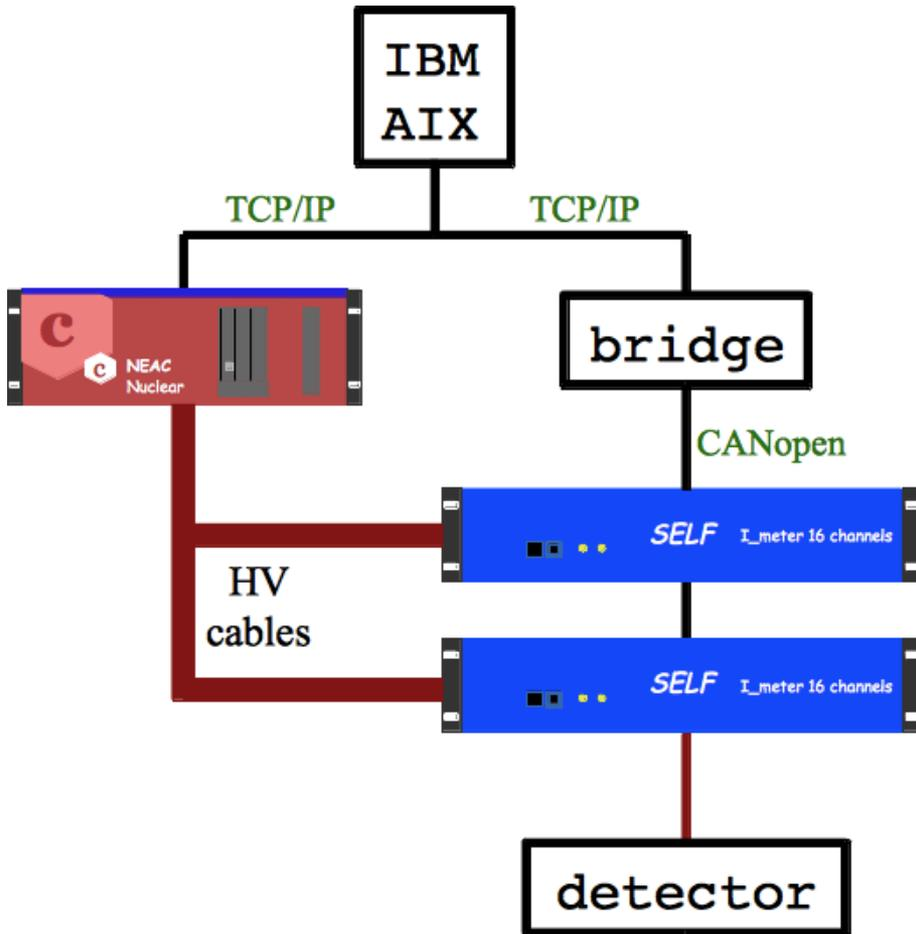
Final HV slow control is being set up
