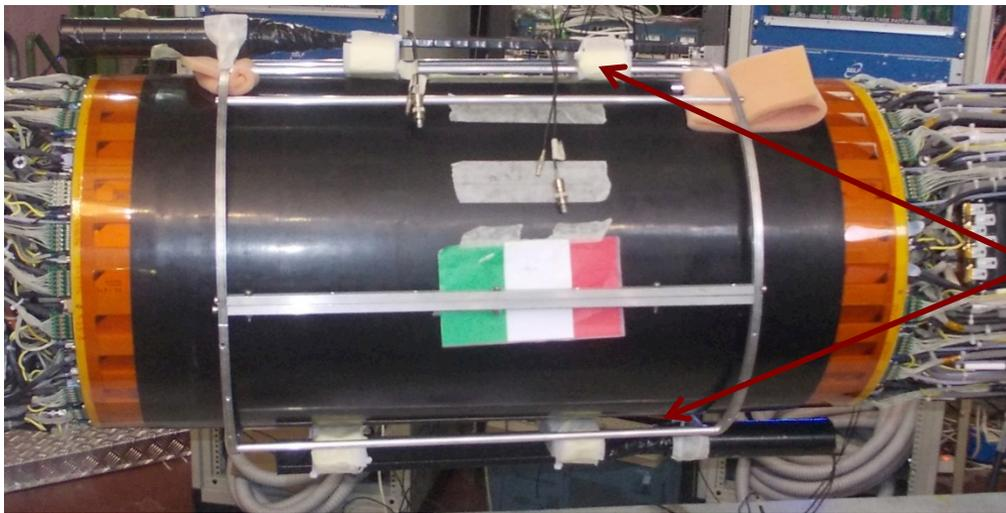
Scintillators for cosmic-ray trigger mounted on a cylindrical rotating support for acquisition on different sectors of the Inner Tracker
