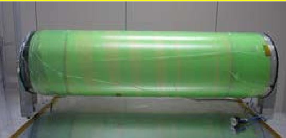
The large electrode is then rolled on a Teflon machined mould, glued and polymerized with the vacuum bag technique
