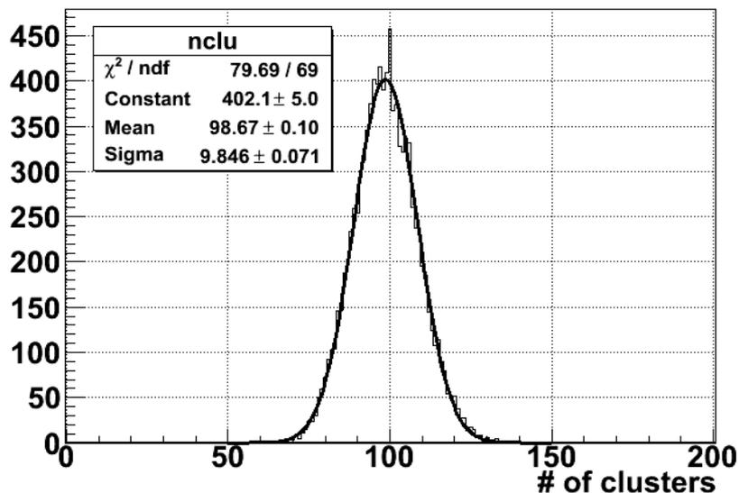
Ionization in 3 mm Ar:isoC<sub>4</sub>H<sub>10</sub> 90:10,  $\beta\gamma=2.21$
