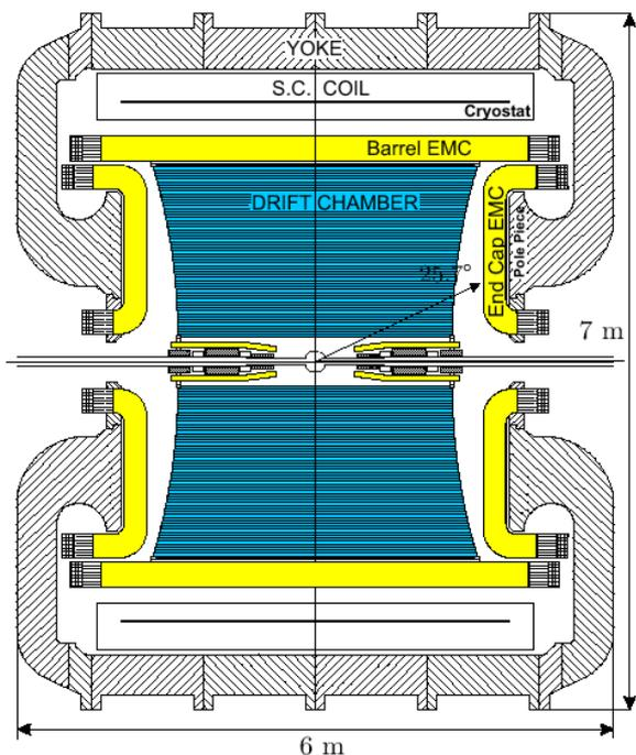
The KLOE apparatus, consisting of a huge **Drift Chamber** and an **Electromagnetic Calorimeter** working in a **0.5 T** axial magnetic field, has been upgraded with new subdetectors (including a **vertex detector**) for a new data taking campaign. The required inner tracker performances are :
