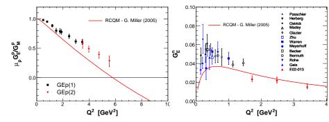
G<sup>p</sup><sub>E</sub> suppression at higher Q<sup>2</sup> due to inclusion of quark orbital angular momentum
