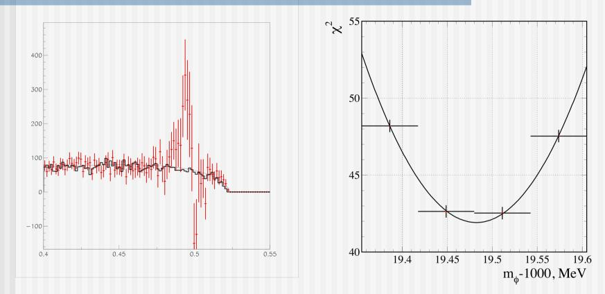
In MC we know all inputs and can create a "test"  $m(K_L)$  distribution and compare with data. And the only free parameter is  $\phi(1020)$  mass. By varying f mass we calculate  $\chi^2$  value by fitting data-MC difference with "ARGUS" function. We obtain:
