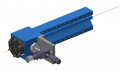
Main Body and Entrance Window made of ASTM B209 AL 7075-T651
