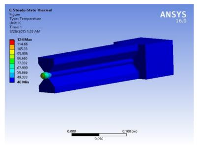
$I_{beam} = 20\mu A$  Max beam current  $A_{raster} = 2x2mm^2$  min raster
