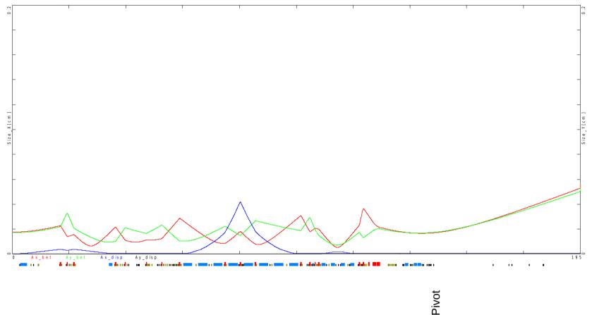
Vertical axis 2 mm, horizontal axis 195 m, Lambertson to dump entrance. Red horizontal size (sigma), green vertical size, Blue dispersion effects (dp/p 0.01%) which must be added in quadrature to red.
