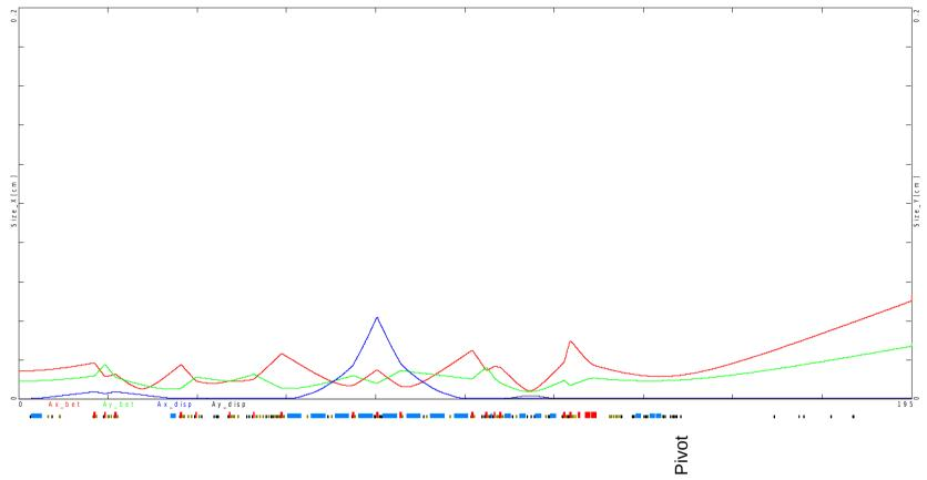
Vertical axis 2 mm, horizontal axis 195 m, Lambertson to dump entrance. Red horizontal size (sigma), green vertical size,
